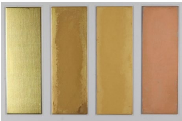
Figure 2: Photographic documentation of brass surface over the test period of 28 days. From left to right 0 d, 1 d, 14 d, 28 d.
