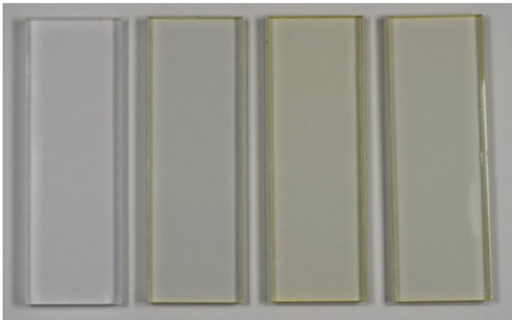
Figure 10: Photographic documentation of polycarbonate surface over the test period of 28 days. From left to right 0 d, 1 d, 14 d, 28 d.
