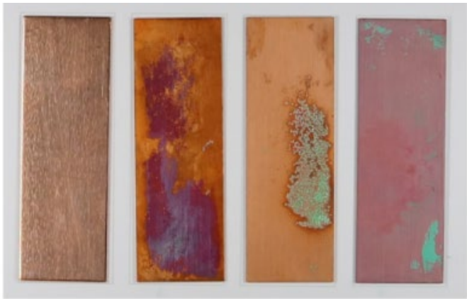
Figure 1: Photographic documentation of copper surface over the test period of 28 days. From left to right 0 d, 1 d, 14 d, 28 d.
