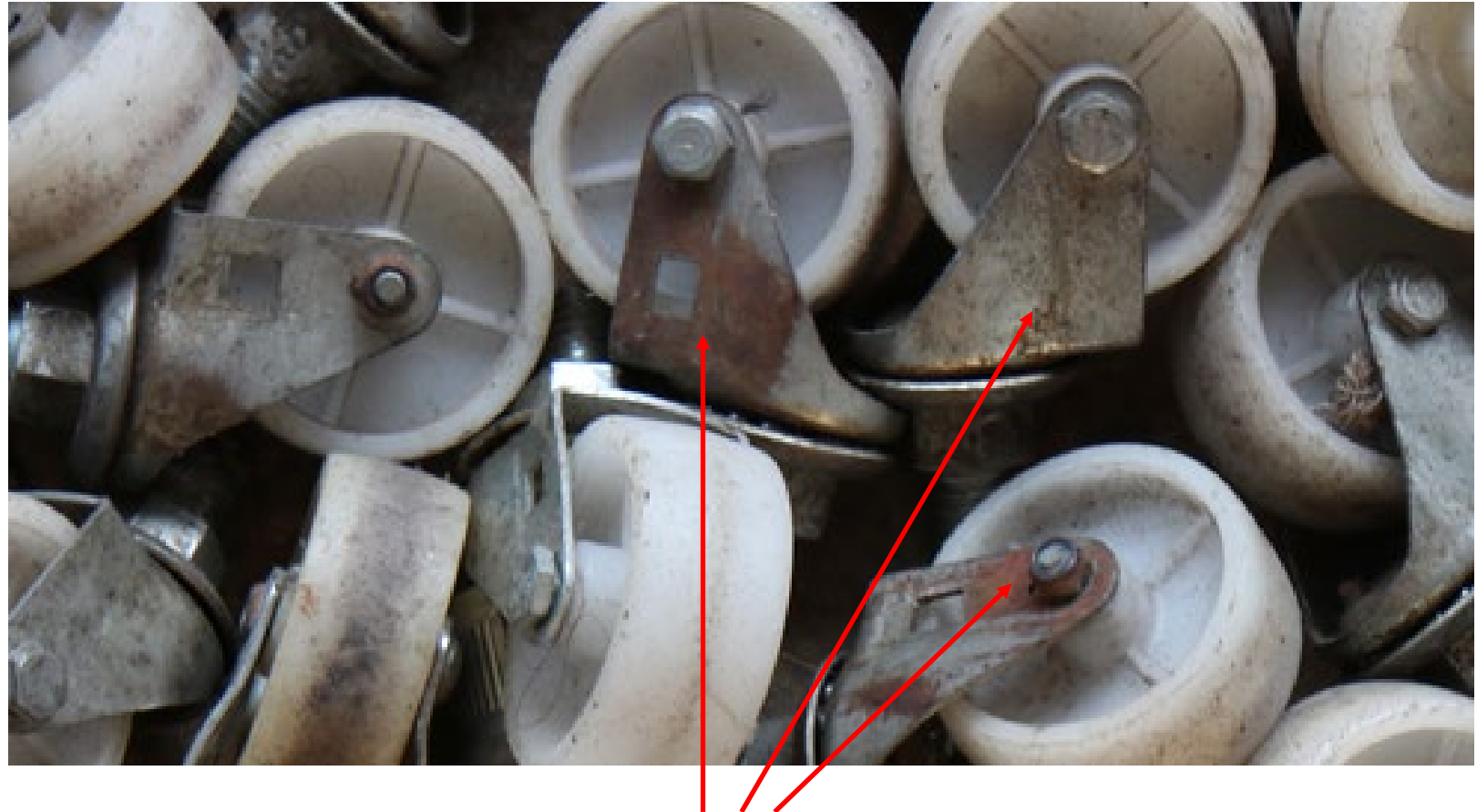
Damages caused by bleach (NaOCl)
