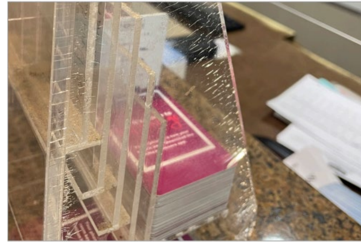
Environmental stress cracking occurs in acrylic after repeated contact with common glass cleaners.
