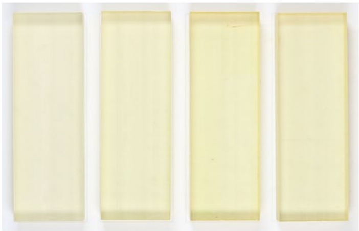
Figure 12: Photographic documentation of polysulfone surface over the test period of 28 days. From left to right 0 d, 1 d, 14 d, 28 d.
